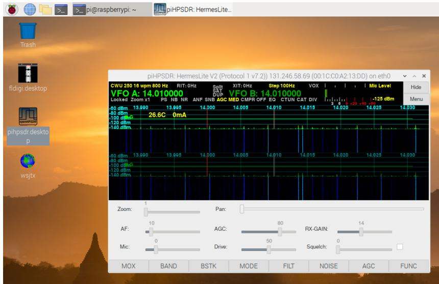
As you can see, the radio starts by default with two receivers, and both receivers have the panadapter and the waterfall on display. This can be configured of course within piHPSPDR and is stored in a local file so the next time you start piHPSPDR, these settings are restored.
