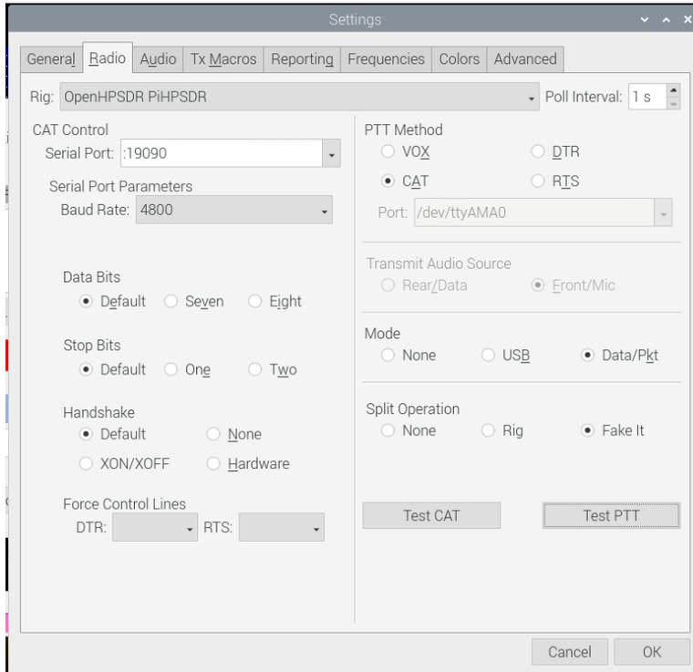
In WSJT-X, go to "File ==> Preferences" and click the "Radio" tab. Choose "OpenHPSDR PiHPSDR" as the rig, enter ":19090" as the serial port (note the colon at the beginning of the string) and enable "CAT" for the PTT method. Choose "Data/Pkt" for the mode (this means that the DIGU mode is chosen in piHPSDR). If you want to TX at audio frequencies below 150 or above 2850 Hz, you also have to choose "Fake It" in the "Split Operation" field.
