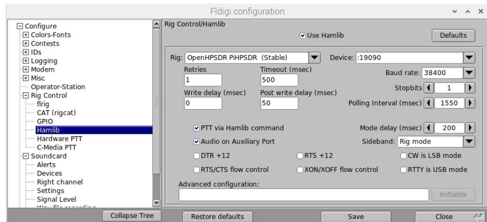
Device (as in wsjtx and as shown in the figure). Then you must check the box at the top "Use Hamlib" and then can hit the "Initialize" button at the bottom right. Do not forget to "Save" the configuration then you can "Close" the window. **When starting FLdigi for the first time, you automatically arrive at the "Hamlib" screen during setup within the FLdigi configuration wizard.**
