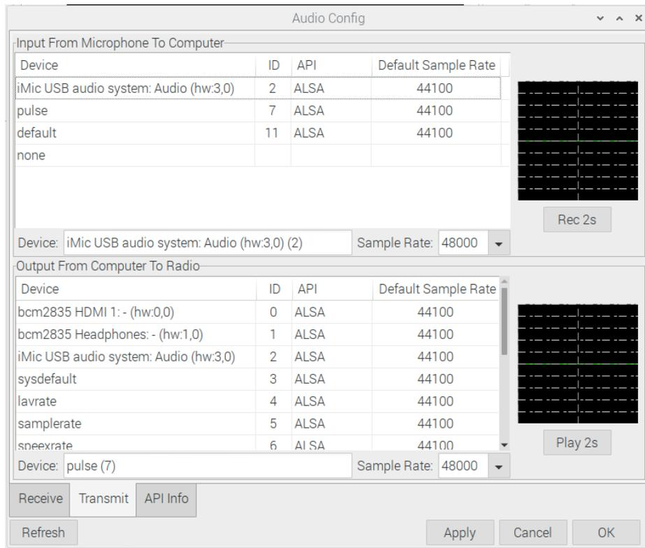
In the "Transmit" tab, choose "pulse" in the "Computer to Radio" section, and the name of your USB sound card in the "Microphone to Computer" section:
