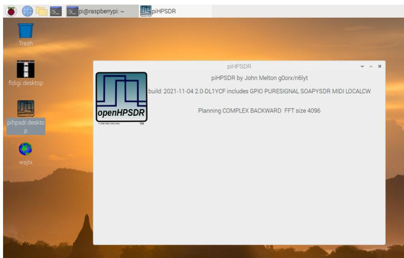
Because it is the first time you started the program, the WDSP library determines (once and for all) the optimum way to do the fast-Fourier-transforms (this will take few minutes, there is a progress report on the screen). After this time, the piHPSDR window looked like this:
