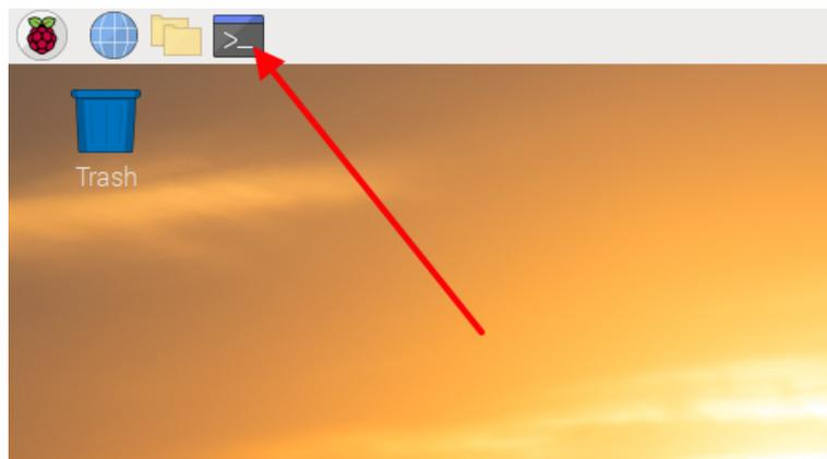
the Raspberry menu Accessoires ==> Terminal. A terminal window opens and looks like displayed in the figure below.
