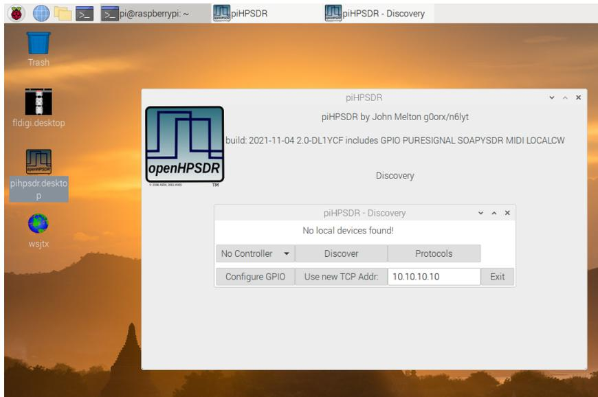
Since we have no radios connected (and therefore no devices have been found), clicking the "Exit" button is the only thing we can do at the moment. If we had connected radios (for example SOAPY devices such as the Adalm-Pluto via USB, or an ANAN radio via an ethernet cable) these devices should be "discovered" and the radio can be started via a "Start" button. In the next picture, this situation is shown, an HermesLite-II has been connected via Ethernet:
