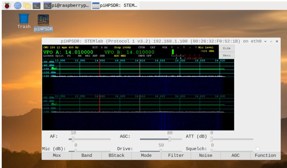
This happens especially when using a large monitor. The reason is, that the system may automatically choose a large font when using a large monitor, which is not reasonable for piHPSDR since it is using a fixed-size window. This is easily fixed from the Raspberry -> Preferences -> Appearance Settings menu, in the window that opens you click the System bar and change the font to a small one, e.g. FreeSans with font size 10. Then immediately the piHPSDR window looks OK.
