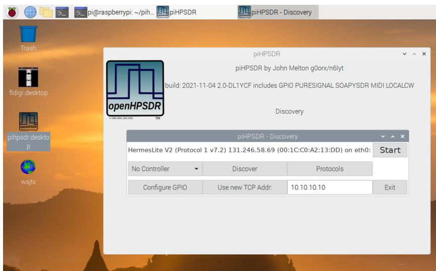
It takes some time to arrive here, because piHPSDR tries to "discover" HPSDR protocol1, HPSDR protocol2, and SoapySDR devices. Using the "Protocols" menu by clicking the tab with that name, one can disable those protocols for which no hardware is present. Clicking the "Start" button then leads to the following
