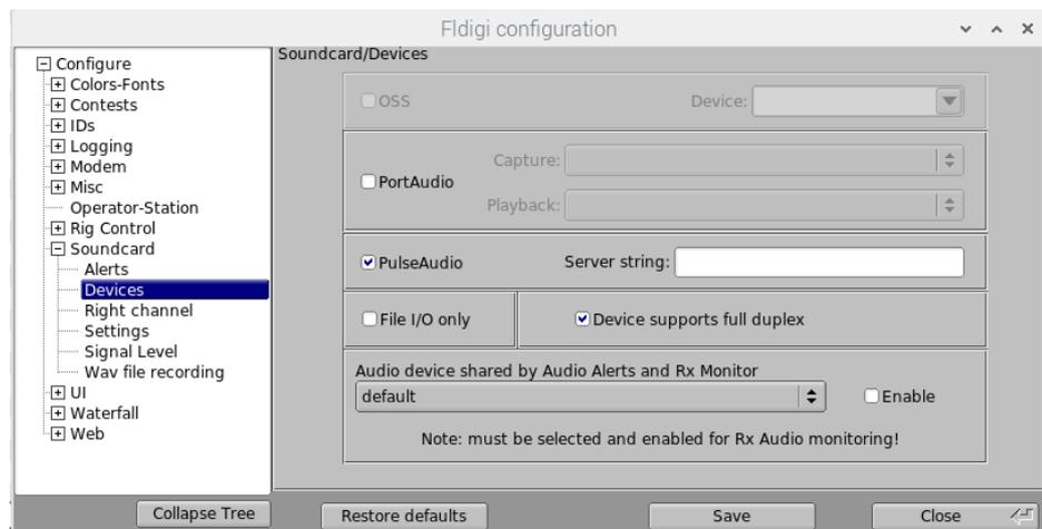
When starting Fldigi for the first time, you automatically arrive at the "Soundcard/Devices" screen during setup within the Fldigi configuration wizard.
