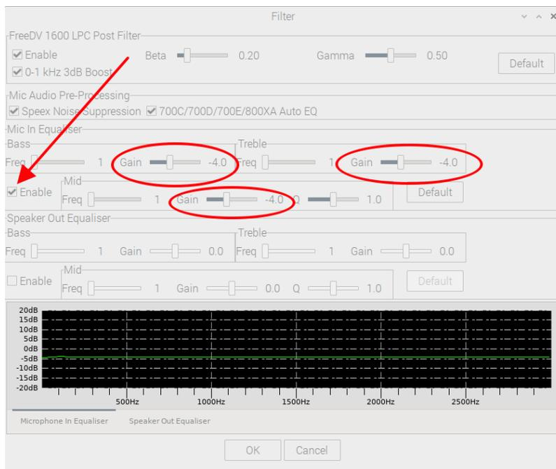
To correct this, go to the Tools ==> Filter menu. There you can enable the mic equalizer (red arrow) and choose the levels for "Bass", "Mid", and "Treble" (red circles). For the default center frequencies (all 1 Hz) only the "Treble" slider has much effect, to achieve a frequency-independent attenuation (see green curve at the bottom) set all three sliders to the same value (-4 dB in my case).
